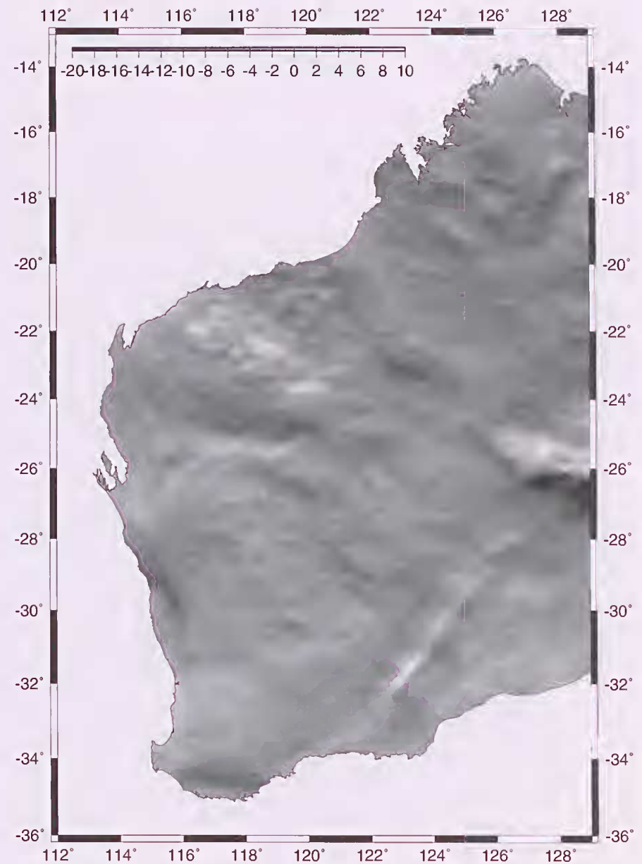
Figure 4. Computed AUSGeoid98 north-south vertical deviations across Western Australia (Mercator projection; Units in arc-seconds).
